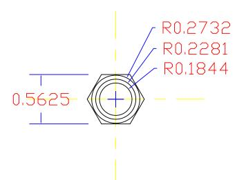
6061 Aluminum Body 302 Stainless Steel Spring Stainless Steel Ball 440 Grade 200 303 Stainless Steel Seat
