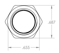
Max. Operating Pressure - 1200 psi Max. Operating Temperature - 180F Seat Area Open Diameter - .280
