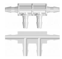
High pressure barb style double branch tee connector. Barb sizes include 1/16", 3/32" and 1/8". Materials include white nylon and natural polypropylene. The **High Pressure Barb Style (HP)** offers outstanding performance characteristics when used with flexible tubing. Tubing is expanded by 50% above its nominal ID, permitting high-pressure capabilities.
