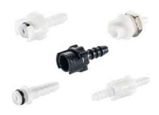
These 1/16" flow size couplings are produced in a natural Acetal (POM) thermal plastic. They are resistant to most mild chemicals and are manufactured to be trouble free for many years of service. They are intuitive to use and make an audible click when coupled. 10AC couplings interconnect with all other 10PP Series couplings as well as other similar industry twist lock type couplings. BLK denotes part available in Black.
