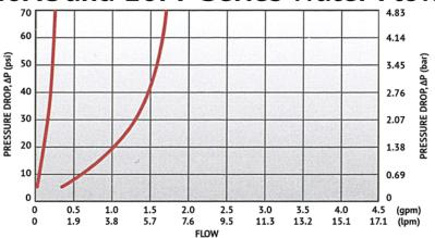
Specific coupling be determined by using this  $|C_v| = Average$  flow rate (see chart) formula:
