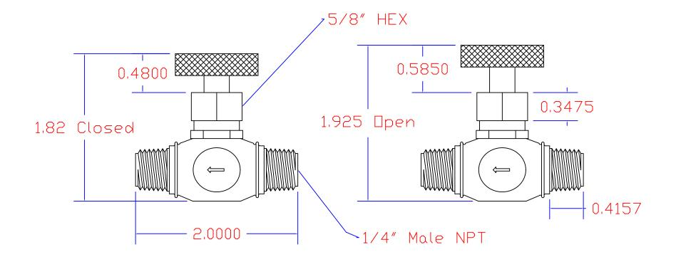
Made of heavy duty brass. This precision valve has a stainless steel stem, tapered to allow accurate micro control of air, liquids and gases that do not affect brass. 125 psi working pressure.
