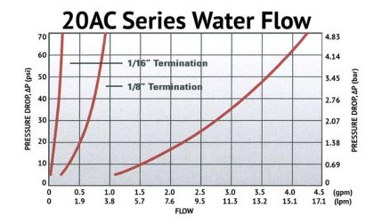
Specific coupling be determined by using this  $C_v = Average$  flow rate (see chart) formula:
